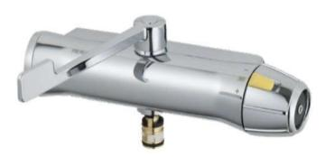
This mixer is a premium point-of-use pressure balanced TMV for basins with a 170mm long lever action headwork, making it perfect for application in hospitals and aged care facilities.
