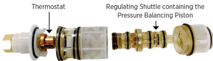
PBTMV Cartridge Exploded View
